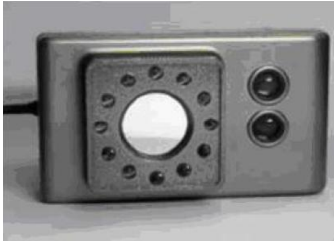
Fig.2 The hand-held iris camera CASIA-IrisCamV2 used for collection of device2
