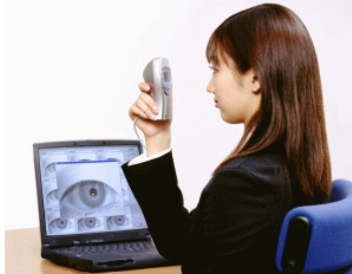
Fig.3 The hand-held iris camera used for collection of CASIA-Iris-Lamp
